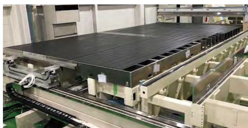
大型基板用气浮式工作台 Float-type stage for large substrates
